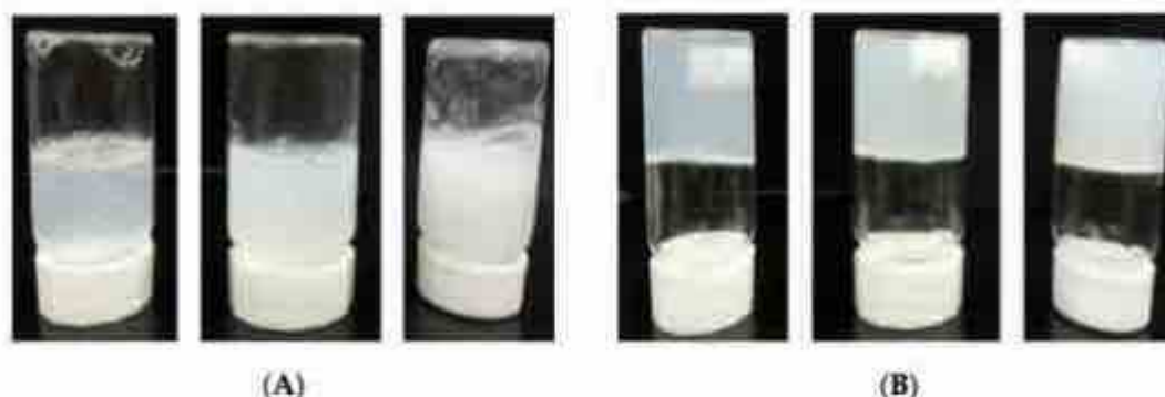
Figure 1. Photographs of the state of the N -Palmitoyl-Glycine-Histidine (Pal-GH) gel formulation in the bottles. The bottles were placed in an inverse position immediately (A) and 5 min after (B) shaking. The Pal-GH concentrations are, from left to right in both photos, 2.5%, 5%, and 10%.
